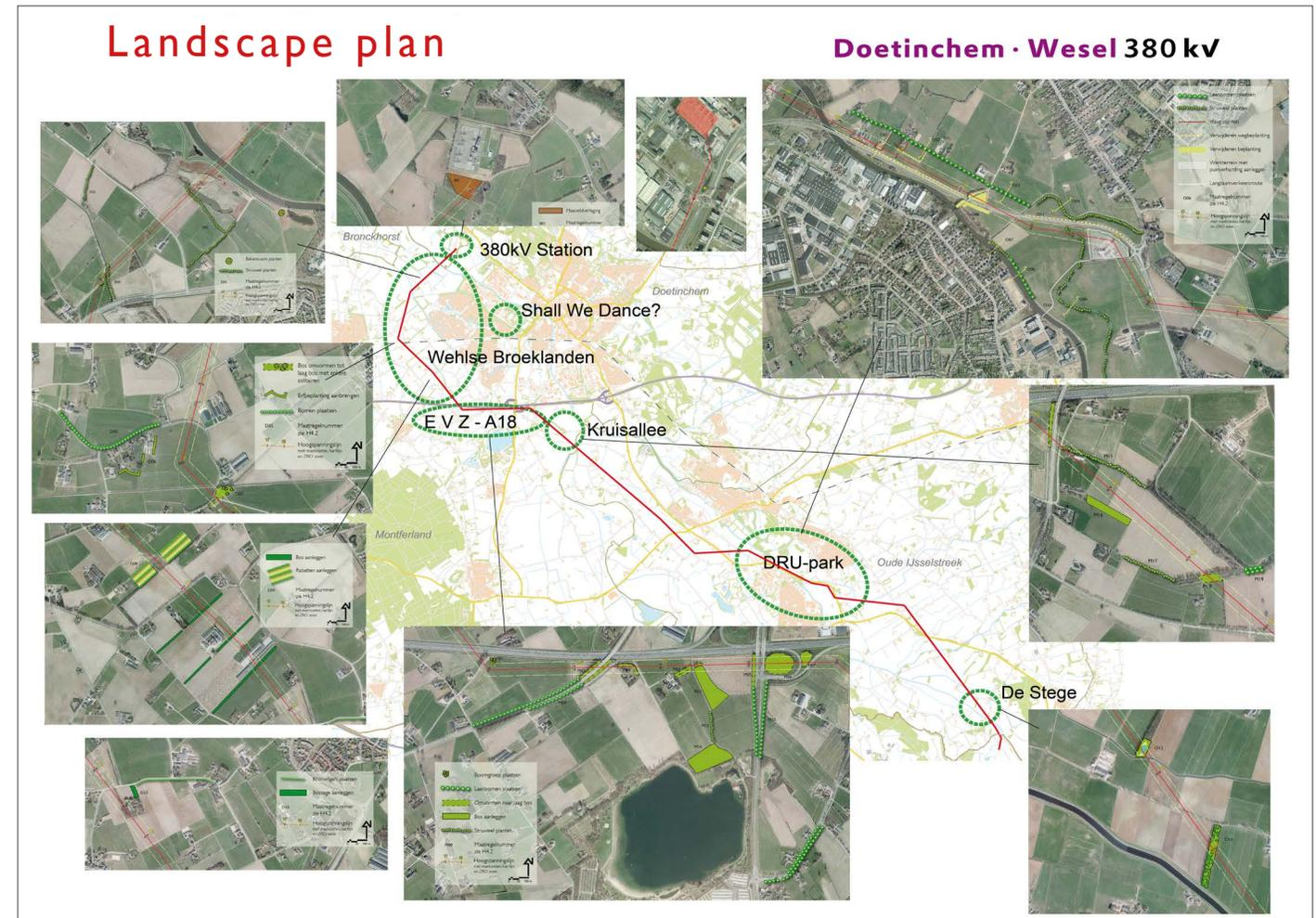
The aim of the design measures included in a landscape plan is to mitigate and compensate for the effects of a new power grid element, such as an overhead line.
