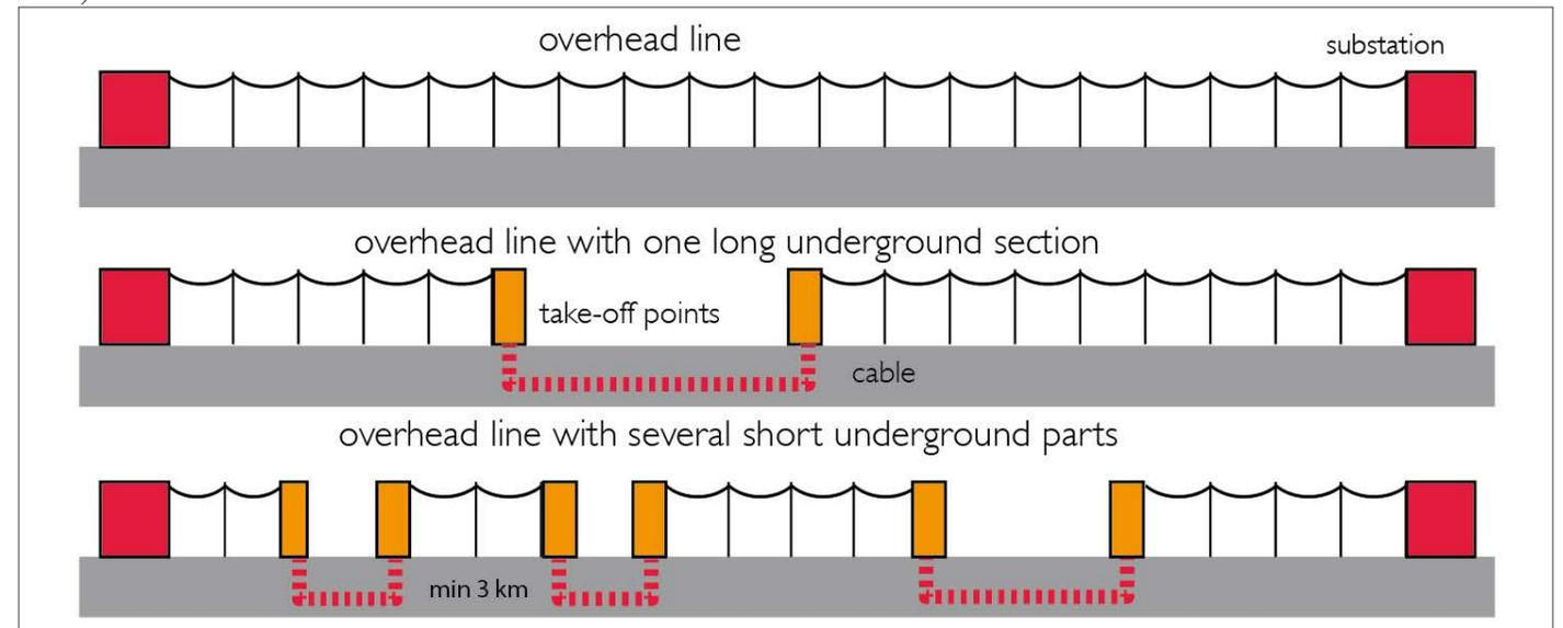
deviation' comparable to the use of extra high masts when crossing a river or channel with a large vertical clearance. The interruption of the overhead line and the transition point strongly determine the appearance of a connection. It is important that there is a recognizable correlation between the use of shorter cabling sections and the functional reason for this in the landscape.
